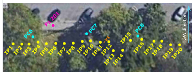
Fig. 3 Injection points and groundwater flow
