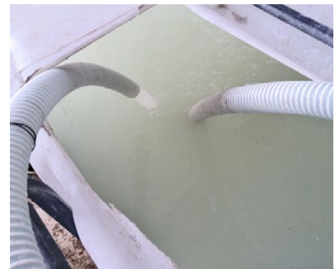
Fig. 1 Petrofix in mixing tank. Equipment used is made of chemically resistant materials.
