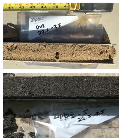
The photo on the top shows a soil core collected before a PetroFix application.
