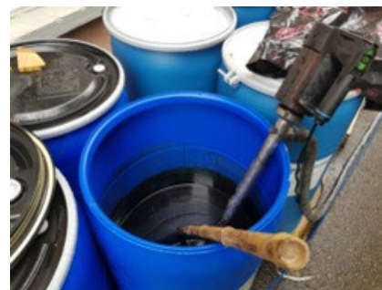
Fig. 3: Drum pump for transfer of PetroFix from drum to mixing tank
