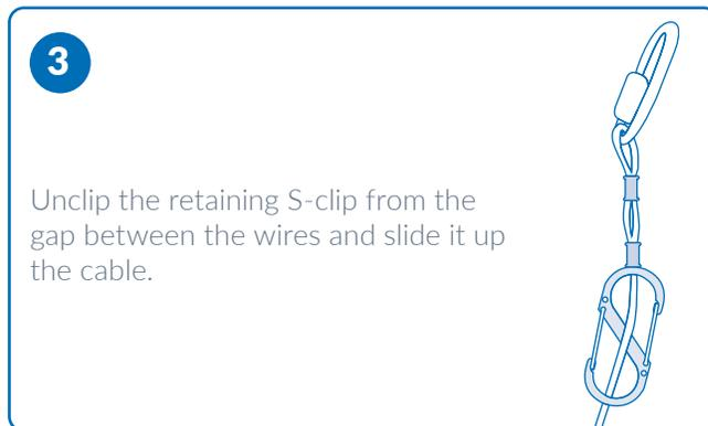
Unclip the retaining S-clip from the gap between the wires and slide it up the cable.
