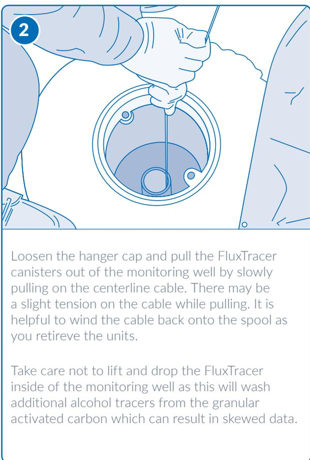
Loosen the hanger cap and pull the FluxTracer canisters out of the monitoring well by slowly pulling on the centerline cable. There may be a slight tension on the cable while pulling. It is helpful to wind the cable back onto the spool as you retrieve the units.
