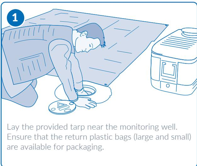
Lay the provided tarp near the monitoring well. Ensure that the return plastic bags (large and small) are available for packaging.
