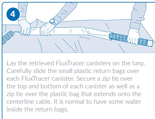
Lay the retrieved FluxTracer canisters on the tarp. Carefully slide the small plastic return bags over each FluxTracer canister. Secure a zip tie over the top and bottom of each canister as well as a zip tie over the plastic bag that extends onto the centerline cable. It is normal to have some water inside the return bags.
