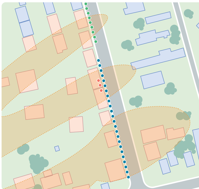
Areal map depicting the location of the three PlumeStop PRB installation phases. Plume boundary shown as it existed prior to application, following discrete sampling of injection wells.
