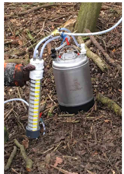
Fig 5 bioaugmentation (BDI Plus) setup for injection
