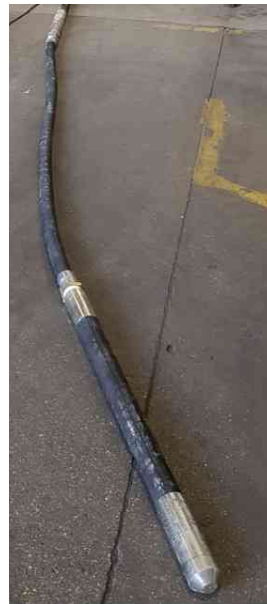
Fig 4 Double packer assembly
