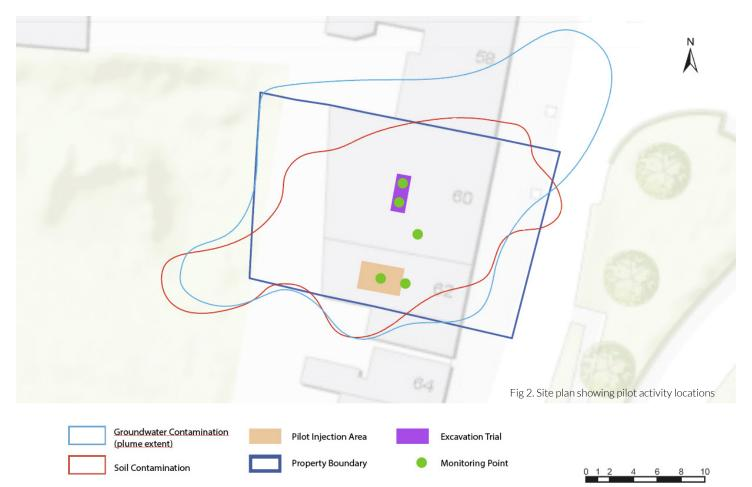
In the centre of the site an excavation application trial was completed. A slit trench was opened up, with the impacted soils segregated for disposal. The base and walls of the excavation were then sprayed with PetroFix to prevent recontamination of clean backfill. The trial also emulated the use of PetroFix in excavation applications to prevent the further advection of the dissolved phase plume in the full-scale project.
