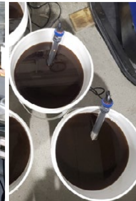
Fig 2. Individual heaters in HRC buckets
