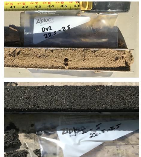
The photo on the top shows a soil core collected before a PetroFix application. The photo below shows a soil core collected after a PetroFix application exhibiting black soil where the PetroFix was successfully distributed
