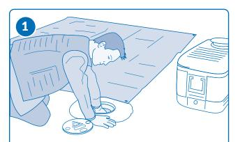
Lay the provided tarp near the monitoring well. Ensure that the return plastic bags (large and small) are available for packaging.
