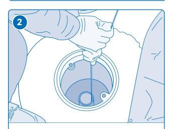
Loosen the hanger cap and pull the FluxTracer canisters out of the monitoring well by slowly pulling on the centerline cable. There may be a slight tension on the cable while pulling. It is helpful to wind the cable back onto the spool as you retireve the units.
