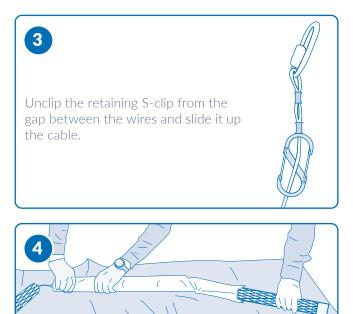
Lay the retrieved FluxTracer canisters on the tarp. Carefully slide the small plastic return bags over each FluxTracer canister. Secure a zip tie over the top and bottom of each canister as well as a zip tie over the plastic bag that extends onto the centerline cable. It is normal to have some water inside the return bags.
